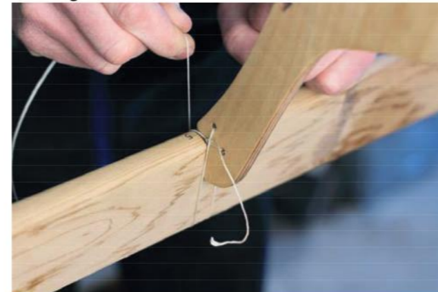
7 - Laying the sinew
