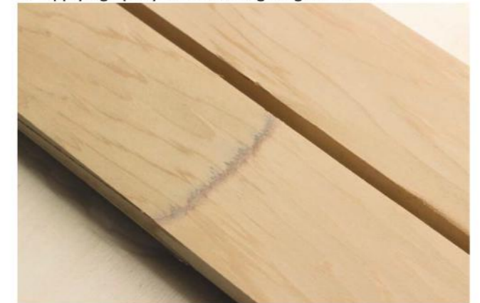
6 - The taper after sanding
