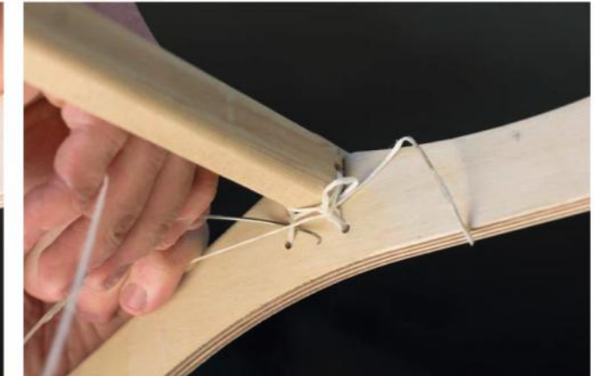
4 - Laying the sinew and tightening the knot
