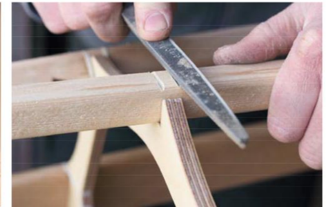
2 - Sinking the sinew into notches
