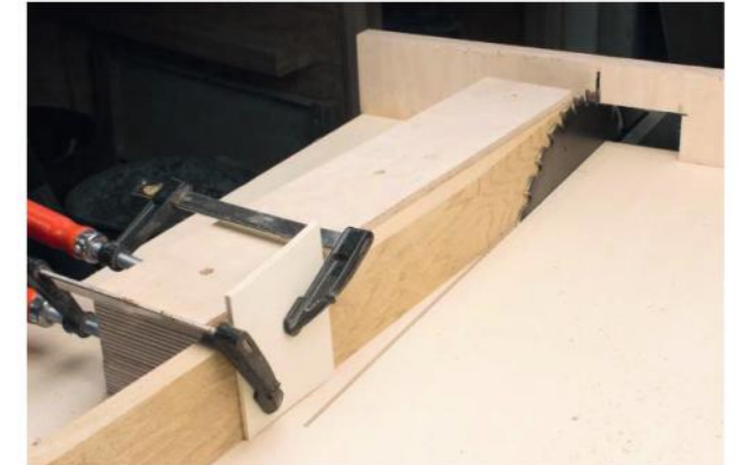
2 – Sawing the tapers
